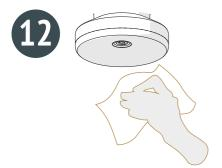
After each pour wipe the rubber head gasket with **FOOD SAFE** sanitary wipes.
