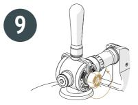
Before releasing the bottle slightly open the drain channel by turning the flow control valve counterclockwise. The pressure in the beverage container takes approximately 10 s to even out with atmospheric pressure.
