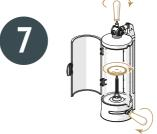
Screw the bottle tray on the end of the shaft with a backing plate on it as well as the handles to the appropriate locations.
