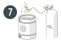
Ensure that the gas cylinder reducing valve is set at a pressure of 1 bar (15 psi). Connect the intake head to the flush keq.
